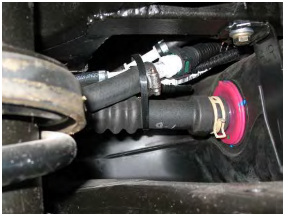
ROLLX VANS HOSES CONNECTING TO OEM HOSES NEAR FUEL TANK
