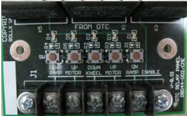
Inputs that run from OTC Control Board.
