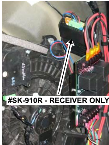
OTC Remote Receiver (Behind Rear Passenger Quarter Panel Above OTC Relay Board)
