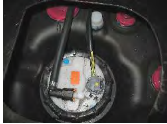
OEM SENDING UNIT (Easily Accessible Behind Rear Sofa on Left Side Under Carpet)
