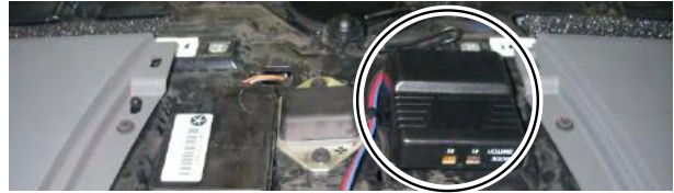
OTC Remote Receiver (After 1/8/2009) (Rear Passenger Quarter Panel)
