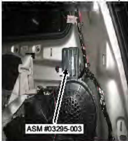
OTC Remote Receiver (Behind Rear Passenger Quarter Panel Above Rear Heat Unit)
