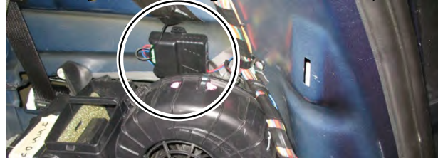
OTC Remote Receiver (After 1/8/2009) (Rear Passenger Quarter Panel)
