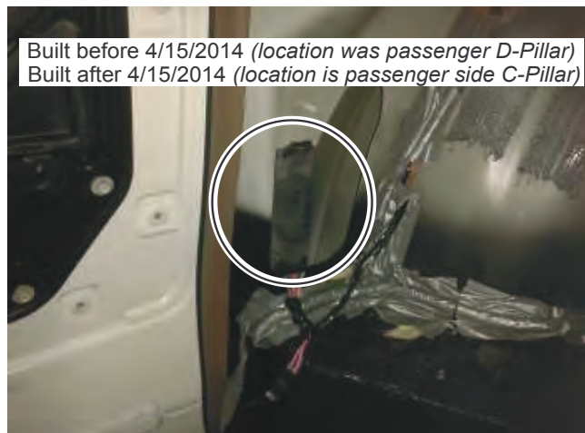
Passenger's Door Detector (Replaced The Door Open Limit Switch after 8/26/2013)
