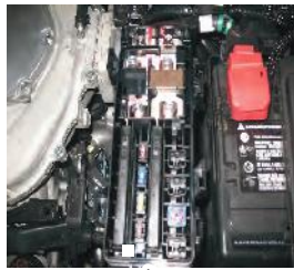
Main Under Hood Fuse Box
