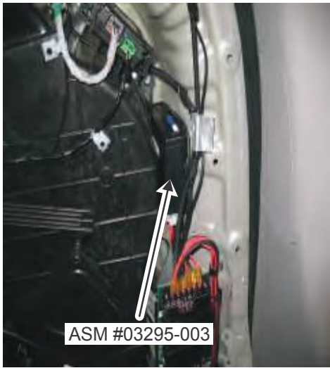
OTC Remote Receiver (Behind Rear Passenger Quarter Panel Above OTC Relay Board)
