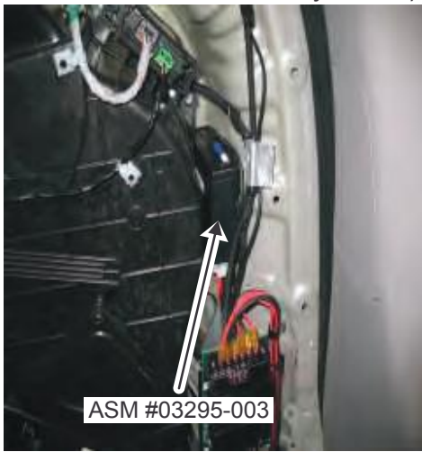
OTC Remote Receiver (Behind Rear Passenger Quarter Panel Above OTC Relay Board)
