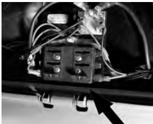
Remote Fuse Box Under Glove Box
