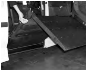
Manual Operation of Ramp
