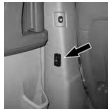
Ramp Override Switch (Location 2)
