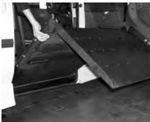
Manual Operation of Ramp
