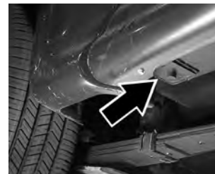
Back Jacking Point
