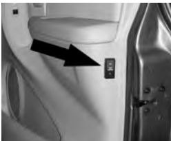
Ramp Override Switch
